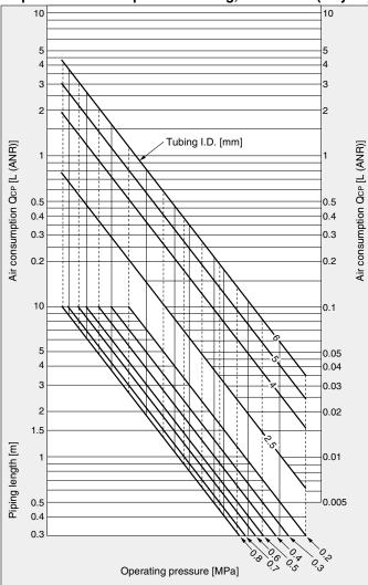
Graph 8 Air Consumption of Tubing, Steel Tube (1 cycle)
