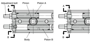
1. It consists of a rack that slides in 2 parallel cylinders, 2 pistons that are integrated with the rack, and a pinion.
