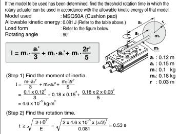
It is therefore evident that there will be no problem if it is used with a rotation time of less than 0.53 s. However, according to the table above, the max. value of rotation time for stable operation is 2 s. Thus, the rotation time should be within the range of  $0.53 \le t \le 2$ .
