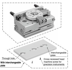
\* To position the product, use the knock pin holes on the body instead of the through holes that are empty in the interchangeable plate.
