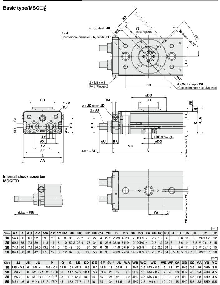
\*1 SU dimension is not the dimension at the time of shipment, since its dimension is for adjustment parts.
